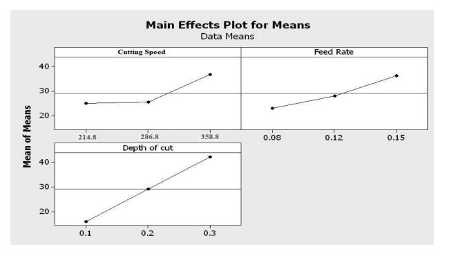
Figure 4.Main effect plots for SN ratio and mean data (MRR)
