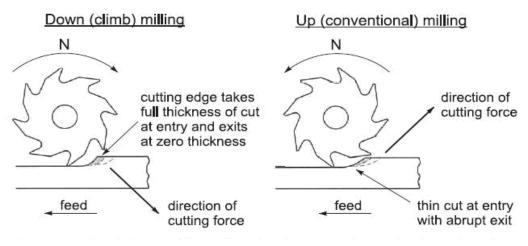
fig.3 types of milling process
